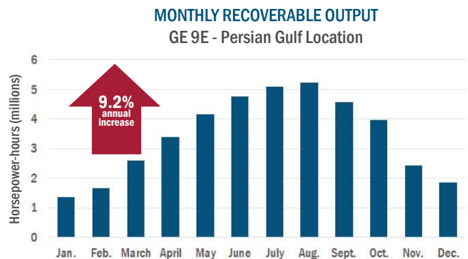
Figure 4: Similarly here, an inlet temperature of 15°C (59°F) will result in a recovery of 9.2% annual horsepower-hours. Calculations are based on Ras Laffan weather data.
