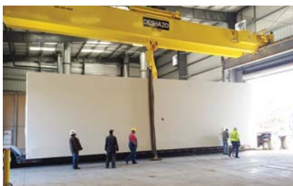
Pictured, top left: The three chiller plants consist of 18 factory-built modules that were custom-designed, pre-engineered and fabricated in a controlled, ISO-certified environment. Modular fabrication enabled a 50% reduction in construction time. Bottom left: Packaged in an enclosed, climate-controlled skid, the modules were pre-piped, wired, tested and shipped to site. Right: All three modular chiller plants (labeled in the photo above) were reassembled on site (image source: www.cheniere.com ).
